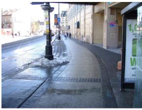
A bus stop detectable strip extends through the sidewalk from shore line to the curb at the bus stop. Street name plates are placed in the sidewalk at all corners of an intersection indicating the name of the street perpendicular to the direction of travel.
