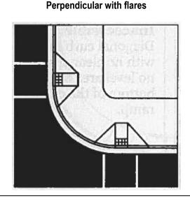
Acceptable design: two parallel curb ramps on a wide turning radius—fit narrow sidewalks
