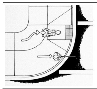
Best design: On small radius corners, curb ramp can be aligned with crosswalk and be perpendicular to curb
