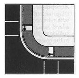
Acceptable design: two combination curb ramps on a corner with a wide turning radius—fit narrow sidewalks; parallel ramp lowers the elevation of the landing and the perpendicular ramp bridges the remaining elevation to the roadway
