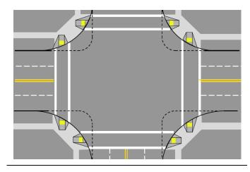
The Ontario Traffic Manual (Book 15 Pedestrian Crossing Facilities) introduces the ladder crosswalk marking: the transverse crosswalk lines are enhanced with longitudinal stripes aligned perpendicular to the pedestrian direction of travel as illustrated in Exhibit 5-10. The larger shapes and tonal contrast of the marking on asphalt increases the visibility of the crosswalk to motorists, in particular, since they see them from a low angle of about 1 m above the ground.
