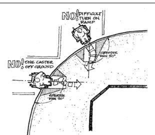
Curb ramps aligned with crosswalks are effective in orientating users to the crossing
