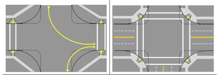
With large corner radii, balance goals for length crosswalk, two separate curb ramps, crosswalk setback and overall walking distance.
